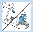
1 Pull the milk container lever upwards with your finger to release the milk container unit. Then pull the milk container unit forwards to remove it from the machine.
