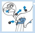
3 Press the milk container lid release lever (1), tilt the milk container lid slightly (2) and pull the milk container lid upwards to remove it from the milk container (3).
