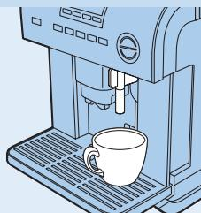
**3** Press the button for hot water until the message 'PROGRAM TO SET VOL - HOT WATER' appears on the display and then release it.
