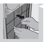
2 To remove the pre-filter, grab the two projections and pull the filter towards you.
