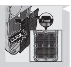
7 Put filter 1 (pre-filter) back into the appliance.
