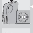
The power-on light, the AUTO light, and the AIR QUALITY light on the control panel go on.
