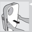
1 Place your fingers in the recesses of the side panels and gently pull the top part of the front panel towards you. Then lift the hooks at the bottom of the panel out of the bottom of the appliance.
