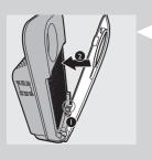
**5** To reattach the front panel, insert the bottom hooks into the bottom of the appliance first (1). Then push the panel against the body of the appliance (2).
