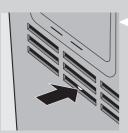
10 Press the filter reset button with a thin tool.
