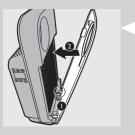
**6** To reattach the front panel, insert the bottom hooks into the bottom of the appliance first (1). Then push the panel against the body of the appliance (2).
