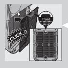
4 Put the pre-filter back into the appliance. Attach all hooks properly to the appliance.
