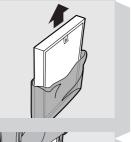
4 Put filter 2 (high-efficiency formaldehyde removal HEPA filter) into the appliance.
