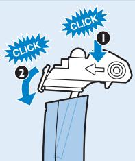
5 To fasten the milk container lid onto the milk container, first push the front of the milk container lid onto the edge of the milk container ('click') (1) and then push the rear end onto the milk container ('click') (2).
