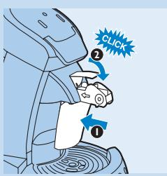
6 Slide the milk container unit into the coffee machine (1) and push down the milk container lever ('click') (2).
