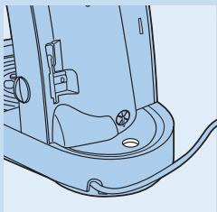
**9** Clean the water inlet on the machine with a moist cloth.
