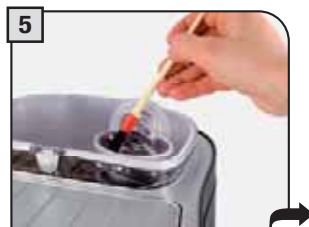
5 With the brush, clean the pre-ground coffee compartment.
