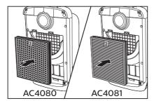
4 After the pre-filter is put back in the appliance, reset the filter 2 lifetime counter. (Refer to chapter 7 "Resetting the filter lifetime counter")
