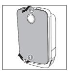
2 To remove the pre-filter, press the two clips down and pull the filter towards you.
