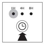
2 Press the timer button (a) repeatedly to choose the number of hours you want the appliance to operate. The corresponding timer light goes on.
