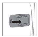
3 Clean the sensor, the dust inlet and the dust outlet with a lightly moistened cotton swab.
