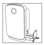
2 Remove the humidification filter from the water tank.
