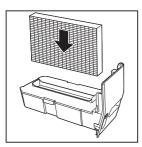
Push the water tank back into the appliance.
