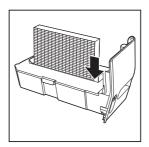
9 Put the water tank back into the appliance.
