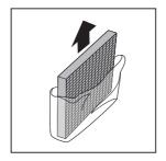
2 Pull out the water tank from the side of the appliance.
