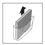
3 Put the new humidification filter in the water tank.
