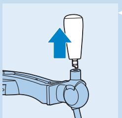
**5** You can remove the tap handle by pulling it out of the tap body.
