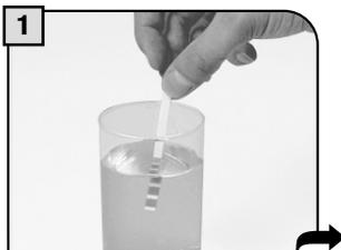
Immerse the water hardness test strip in water for 1 second.
