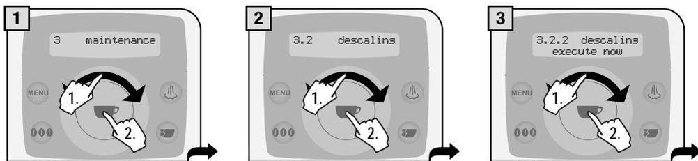
Descaling is performed at a controlled temperature. If the machine is cold, you must wait until it has reached the right temperature; otherwise you must cool the boiler as follows:
