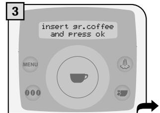
A message reminds the user to insert ground coffee into the appropriate compartment.
