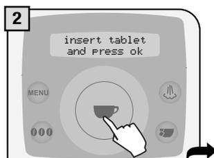
Insert the cleaning tablet as shown above. Press
