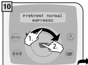
Change the prebrew value (normal, long, off) by turning the click wheel with your finger. Press the
