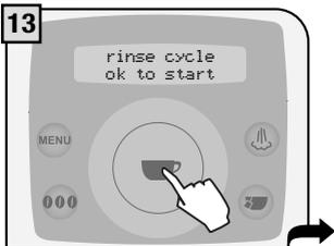
Rinse the machine's circuits by pressing the
