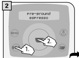
Select the function by pressing the **000** button until the pre-ground option appears. Press the
