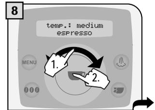
Change the temperature setting (high, medium, low) by navigating the click wheel with your finger. Press the
