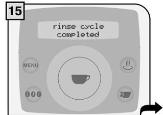
When the rinse cycle is finished the above screen appears. Then the display shows the maintenance screen.
