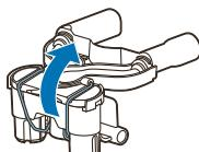
6 Remove the inside part of the frothing system by pulling it downwards.
