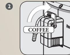
2 Push the lever to the up position to select the COFFEE function.
