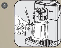
4 Place a container under steam wand. Press the “☕” button to start the cycle. The machine will start the automatic priming by dispensing some water through the steam wand. When the machine stops dispensing, a warm up cycle will begin automatically.
