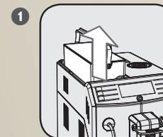
Open lid and use handle to remove water tank. To use without water filter, rinse tank with water. Fill with fresh water up to MAX mark. Place water tank into machine. To install water filter see user manual.
