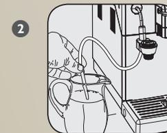
2 Plunge suction tube into a milk container. Place a cup under the automatic milk frother. Press the “☕” button then press the “☕” button to start dispensing frothed milk. Frothed milk will continue to dispense for 3 minutes or until you press the “☕” button to stop dispensing.
