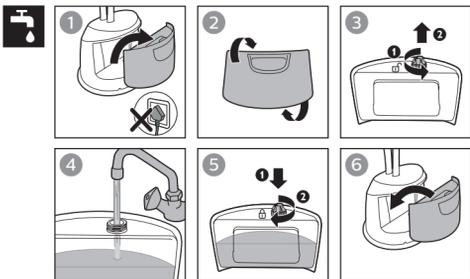
**EN** Your appliance has been designed to be used with tap water. In case you live in an area with hard water, fast scale build-up may occur. Therefore, it is recommended to use water without minerals such as distilled or purified water to prolong the lifetime of your appliance.
