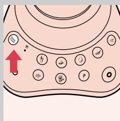
**1** Pour lukewarm water and some washing-up liquid into the blender jar, up to 1/2 of the jar. Do not exceed this level when using the Quick Clean function.
