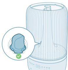
4 Fill the water tank with water. Do not fill with hot water.
