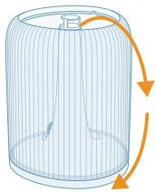
8 Remove the deafener from the bottom of the water tank.
