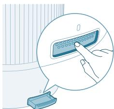
**2** Remove the aroma pad and rinse the pad and the box under warm, running water.
