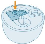
**13** Put the water filter back to the water tank.
