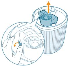
9 Remove the float from the base chamber.
