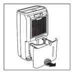
3 Open the water tank cover and fill the water tank for 1/3 with water.
