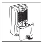
2 Open the water tank cover and empty the water into a sink.
