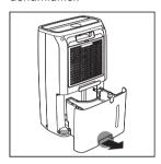
3 Connect the hose to the drainage outlet.
