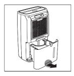
Open the water tank cover and fill the water tank for 1/3 with water.
