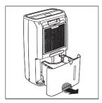
Open the water tank cover and empty the water into a sink.
