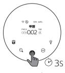
3 seconds to switch off the air purifier.
