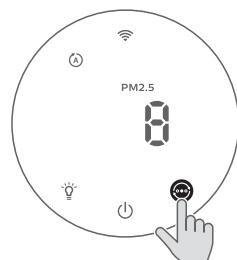
**Auto mode (A):** The air purifier automatically adjusts the fan speed in accordance with the ambient air quality.
