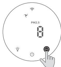
**Manual speed (S1 & S2):** In manual mode, the air purifier operates on speed 1 or speed 2.
