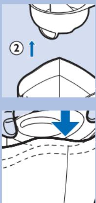
Make sure that the deflector and the filter have been inserted into the dust compartment before using the appliance to suck up either dry materials or liquids.
