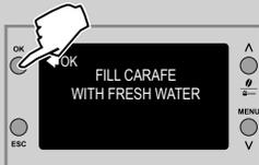
**14** Wash the milk carafe thoroughly and fill it with fresh water. Insert the milk carafe into the machine. Press the “OK” button to confirm.
