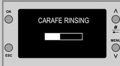
**16** The machine starts dispensing water from both the coffee and the milk dispensing spout. The bar shows the cycle progress.
