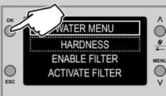
**7** Select HARDNESS option by pressing the "OK" button and set the water hardness value.
