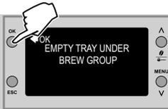
**10** Empty the (internal) drip tray and place it back. Then, press the “OK” button.
