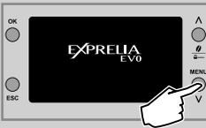
**4** Now you can program the water hardness setting. Press "MENU" button to access the machine main menu.
