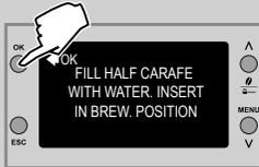
**11** Empty the milk carafe and fill it with fresh water. Insert it back in the machine. Press the “OK” button.
