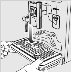
**4** Attach the drip tray (external) with grill to the machine. Make sure it is placed correctly.
