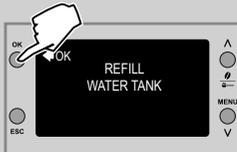
**12** When the machine stops dispensing, fill the tank with fresh water up to the MAX level. Press the “OK” button to confirm.
