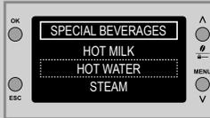
**2** Select **HOT WATER** by pressing the “V” or “^” scrolling button. Press “OK” to confirm.
