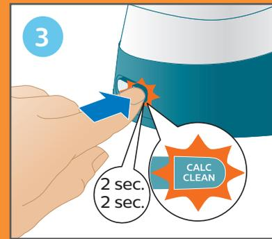
Press and hold the 'CALC CLEAN' button for **2 seconds** until you hear short beeps.
