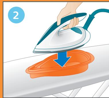
Place the iron on the Calc-Clean container on an even, stable surface.
