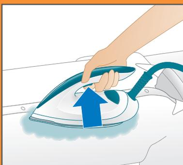
For fast and excellent results, press and hold the steam trigger during ironing. Release trigger to apply a few dry strokes before finishing an area to get the best results.
