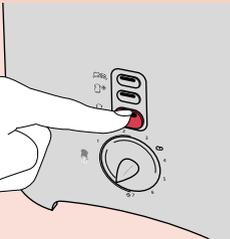
**5** Select the desired browning setting, push the toasting lever down to switch the appliance on and press button
