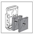
4 Remove all packaging materials of the air purification filters.
