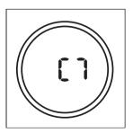
Touch and hold → for 3 seconds to force reset the filter lifetime of the NanoProtect filter AC and exit the filter force reset mode.
