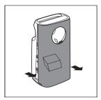
Press the two clips down and pull the pre-filter towards you.
