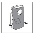
2 Press the two clips down and pull the pre-filter towards you.
