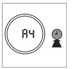
3 Touch and hold → for 3 seconds to confirm the filter code of the new filter
