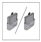
**5** Put the unpacked air purification filters back into the appliance.
