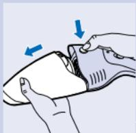
**1** Remove the deflector and the filter frame from the dust compartment.
