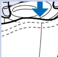
**2** Push the filter firmly into the dust compartment.
