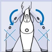
**2** When sucking up liquids, hold the appliance with the dust compartment pointing downwards at an angle. Make sure the squeegee touches the surface to be cleaned. Do not tilt the appliance to one side.
