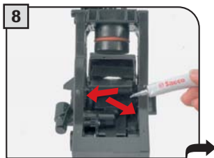
Lubricate the Brew Group guides only with the supplied grease.
