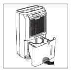
2 Open the water tank cover and empty the water into a sink.
