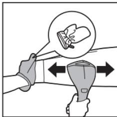
**EN** Put the glove on the hand you are using to hold a garment. The glove protects your hand against the steam from the steamer head.
