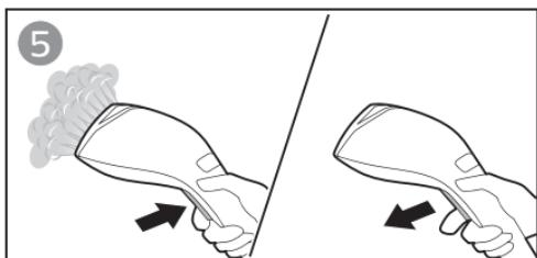
**EN** Press and hold the steam trigger to start steaming.
