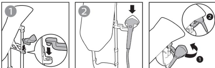
**EN** This side docking allows you to access steamer head conveniently without the hassle of reaching high up. You can choose to use the side docking at either the right side or left side of the device.
