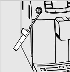
**25** Place the "INTENZA+" water filter (if installed) back in the tank and reinsert the Classic Milk Frother.
