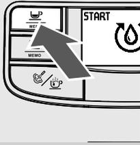
**2** Press the “
