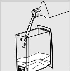
**6** Remove the water tank and pour the entire content of the Saeco descaling solution. Fill the water tank with fresh water up to the MAX level.
