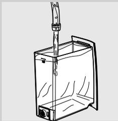
**12** Remove the water tank, rinse it and fill it up to the MAX level with fresh water. Place it back into the machine.
