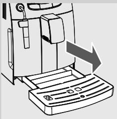
**16** To clean the drip tray, place "Coffee Oil Remover" tablet inside and fill it 2/3rds full with hot water. Let the cleaning solution take effect for about 30 minutes, then rinse thoroughly.
