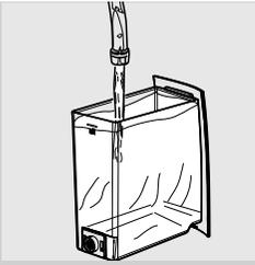
**17** When the water tank is empty, remove it, rinse it and fill it up to the MAX level with fresh water. Place it back into the machine.
