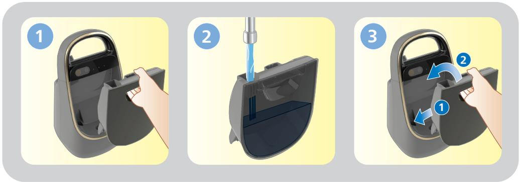
**EN** The appliance is suitable to be used with tap water. However, if you live in an area with hard water, we recommend that you mix an equal amount of tap water with distilled or demineralized water. This will prevent fast scale build up and prolong the lifetime of the appliance.
