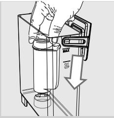
**11** Put the "INTENZA+" water filter into the empty water tank. Press it down until it cannot move any further.
