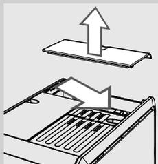
**1** Remove the protection cover from the machine.
