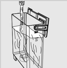
7 Fill the water tank with fresh water up to the CALC CLEAN level. Put the water tank back into the machine. Press the "✓" button.
