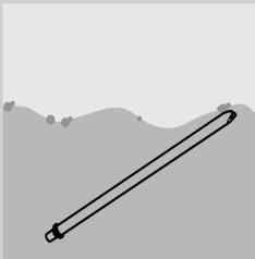
**5** Wash the suction tube with the fitting thoroughly with fresh water.
