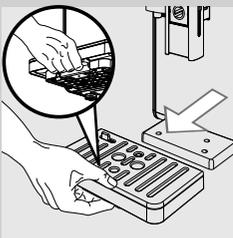
**7** Press the lever on the bottom and remove the drip tray (external), empty it and wash it.
