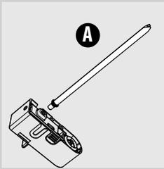
**4** Remove the suction tube with the fitting (A) from the milk frother.
