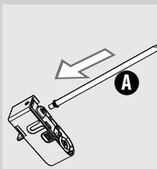
**14** Insert the suction tube with the fitting (A) into the milk frother.
