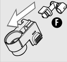
**10** Insert the fitting (F) into the milk frothing device by pressing it up to its limit.
