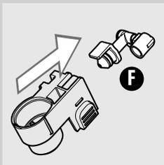
8 Remove the fitting (F) from the milk frothing device by pulling it outwards.
