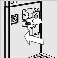
**8** Slightly tilt the water dispensing spout and insert it all the way into the guides of the machine. Push the water dispensing spout towards the bottom while rotating it at the same time, until it is locked into the machine as shown in the figure.
