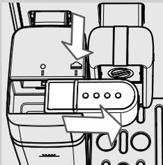
11 Insert the carafe into the machine. Slide the carafe dispenser to the right up to the "☼" icon. Press the "✓" button to confirm.
