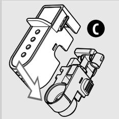
6 Detach the lid (C) from the milk carafe dispenser by slightly pressing on the sides while pushing downwards.
