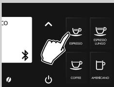
**9** Coffee brewing automatically stops when the preset level is reached; press the same selected beverage button again to stop it earlier.
