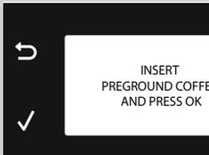
**8** Press the “✓” button. After the prebrewing cycle, coffee begins to pour out of the coffee dispensing spout.
