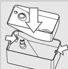
**6** After cleaning and drying the tray, insert it back into the coffee bean hopper. Insert the tray hooks into their seats on the coffee bean hopper.
