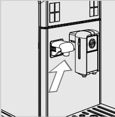
**14** Check that the water dispensing spout is correctly installed.
