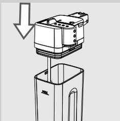
**17** Attach the top of the milk carafe, ensuring it is locked into place.
