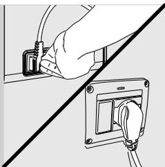
**11** Insert the plug into the socket located on the back of the machine.
