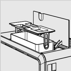
6 Remove the water tank by using the handle incorporated on the inner lid.
