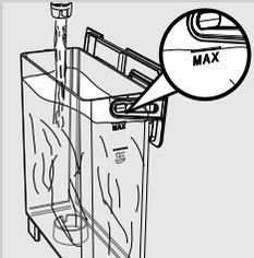
**15** At the end, fill the water tank again up to the MAX level. Now the machine is ready to brew coffee. This icon will be displayed.
