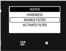
Under **ENABLE FILTER** the machine notifies the user when the water filter needs to be replaced.
