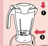
**2** Mount the blender jar on top of the motor unit by turning it in the direction of the arrow until it is firmly fixed. The handle must be facing to the left!
