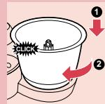
**2 Put the mixing bowl on the motor unit and turn it to the left until you hear a 'click'.**
