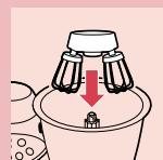
**5 Fit the mixing accessory onto the tool holder.**
