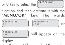
Use the A or V key to select the setting desired and memorize it with the "MENU/OK" key.
