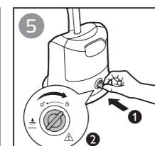
**EN** To maintain optimal steam performance and prolong the lifetime of the appliance, it is important to remove scales and impurities inside the appliance regularly. Therefore, it is recommended to perform the de-calc process at least once a month.
