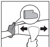
**EN** Put the glove on the hand you are using to hold a garment. The glove protects your hand against the steam from the steamer head.
