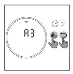
Touch and hold for3 seconds to force reset the filter lifetime counter.
