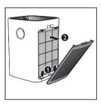
**7** Repeat the above steps and assemble the filter for the other side of the appliance.
