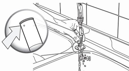
Clean the fixed part installed on the steam / hot water wand with a damp cloth.
