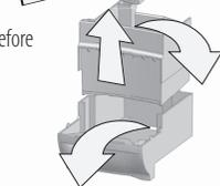
**i** Check periodically that the dregdrawer is not full so as to avoid malfunctioning and damages to the machine.
