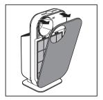
**3** Press the two clips down and pull the pre-filter towards you.
