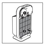
4 Put the unpacked air purification filter into the appliance.
