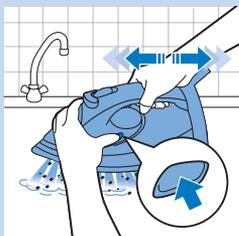
Scales is flushed out, steam and boiling water also come out of the soleplate.
