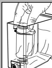
Insert the filter in the empty tank. The reference mark and the groove must match. Push firmly until it is completely inserted.
