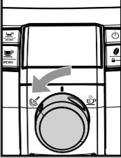
• Turn the selector dial counter-clockwise to set it to the “☁” position. Froth the milk by gently swirling the cup.
