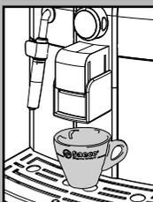
Manually move the dispensing spout up or down to adjust its height by placing your fingers as shown in the figure.
