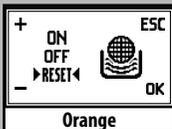
**i** **Note:** When an “Intenza” filter must be replaced with a new one, the function must be reset. Replace the filter as previously shown. After that, enter the programming menu until the indicated window is displayed and select the “RESET” option; then press the “
