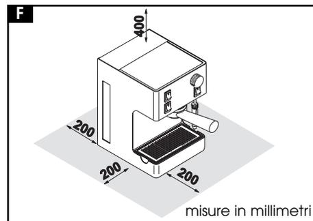
misure in millimetri
