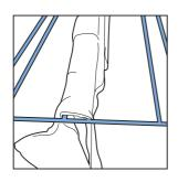
EN Tip: The top rack is only used for hanging garments. It is specially designed to optimize hot air penetration. Drape garments over the rack. Overlapping of garments should be avoided in order to achieve desired result in a shorter time.
