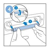
EN Align the pins of the new bulb with the openings of the bulb holder and push the bulb in. Rotate the bulb upwards to tighten it.
