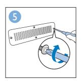
**EN** Put back the metal cover. Insert the rings onto the screws. Tighten the screws on the metal cover.
