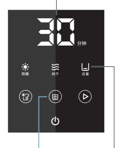
Press the load button to select the desired load.
