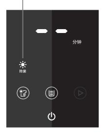
Time display lights up to indicate the pre-set operating time for the selected mode and load.
