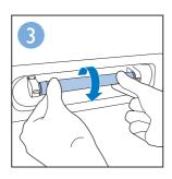
EN Rotate the bulb until the pins on both sides align with the openings of the bulb holder. Pull out the bulb.
