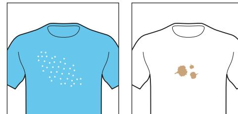
**EN** Over time, impurities in water can form residues in the steam vents and soleplate of the iron. This reduces the steam performance of the appliance and causes white flakes or brown stains coming out of the soleplate. To minimise this, perform the Calc-Clean process regularly.
