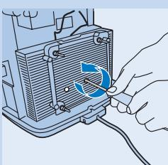
**5 Pull the cooling fan out of the appliance.**
