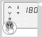
6 Press the temperature up or down button to choose the needed temperature.
