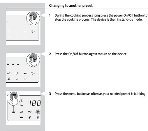
4 Press the On/Off button to start the cooking process.
