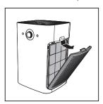
2 To take out the pre-filter, press the two clips down and pull the filter towards you.
