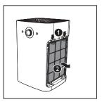
3 Take out the air purification filter from the appliance.
