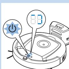
**3** The battery indicator on the display of the docking station and the light in the on/off button on the robot start flashing.
