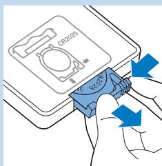
The remote control works on a CR2025 coin-shaped battery. Replace the battery when the robot no longer responds when you press the buttons on the remote control.
