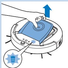
Empty and clean the dust container when the dust container full icon on the display of the robot lights up.
