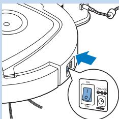
**2** Press the power switch to switch on the robot.
