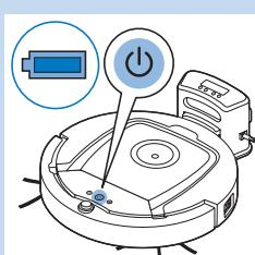
**4** When the rechargeable battery is fully charged, the battery indicator on the display of the docking station and the light in the on/of button on the robot stop flashing.
