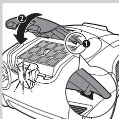
**6** To close the HEPA exhaust filter grille, first align the lugs on the top of the grille with the slots in the appliance (1). Then press the tabs downwards until the grille locks into place (2) ('click').
