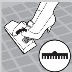
You can use the combination nozzle on carpet (with the brush strips folded in) or on hard floors (with the brush strips folded out).
