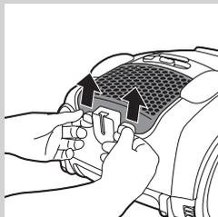
**1** To open the HEPA exhaust filter grille, grab the tabs and pull the grille upwards to remove it from the appliance.
