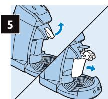
Lift the lever and remove the milk container unit from the machine.
