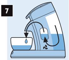
The water in the water reservoir is flushed through the machine and the boiler is filled with water. This process stops automatically, do not interrupt it!
