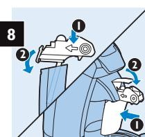
Reattach the lid, place the milk container unit in the machine and press down the lever.
