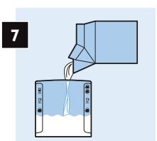
Fill the milk container with cold milk (5-8°C) to the correct level.
