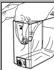
Remove the small white filter from the tank and store it in a dry place sheltered from dust.
