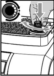
The reference marks inside the coffee bean hopper indicate the grind setting. There are 5 different grind settings to choose from with the following references:
