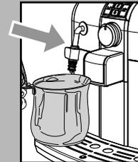
2 Pour the entire content of the Saeco concentrated descaling solution into the water tank and then fill the tank with fresh drinking water up to the MAX level. Place the tank back in the machine.
