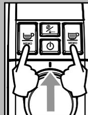
4 Press and hold the 2 brew buttons at the same time for 3 seconds: the descaling cycle is started.
