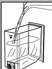
19 Remove the water tank, rinse it and fill it up to the "MAX" level with fresh drinking water.
