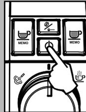
To turn the machine on again simply press the STAND-BY button (if the power button is set to “I”). In this case the machine will go through the rinse cycle only if the boiler is cold.
