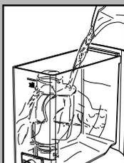
Fill the tank with fresh drinking water and reinsert it into the machine.
