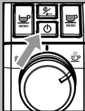
22 When the second rinse cycle is over, the machine enters the stand-by mode and the "☕" button starts blinking.
