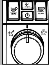
If descaling solution and/or water spills out of the dispensing spout: **PAUSE:** turn the selector dial to the "☕" position; **START:** turn the selector dial to the "0" position.
