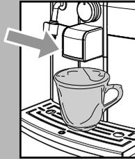
If descaling solution and/or water spills out of the steam wand: **PAUSE:** turn the selector dial to the "☕" position; **START:** turn the selector dial to the "☕" position.
