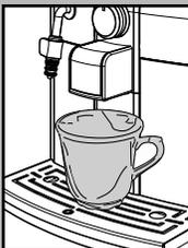
**!** Warning! Remove the "Intenza" filter (if installed) before adding the descaling solution.
