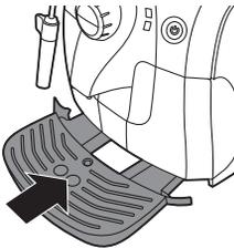
Note: Make sure the drip tray is fully inserted.
