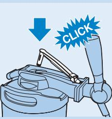
3 Push the tube connector into the opening in the tap unit ('click').
