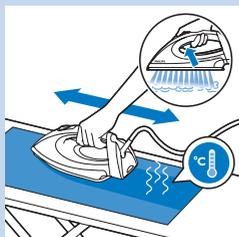
**4** Put a piece of thick cloth on your ironing board. Place your iron on the cloth, press and hold the steam trigger. While pressing the steam trigger, slowly move the iron back and forth across the cloth until no water comes out anymore or when steam comes out.
