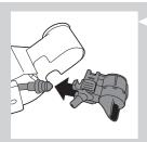
4 Push the milk dispensing spout onto the fitting.
