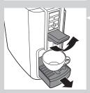
2 For a black coffee or café latte, pull the drip tray to the outer position and pull the coffee dispensing spout up in the horizontal position.
