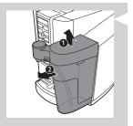
3 To remove the milk carafe, lift it and pull it carefully away from the machine.
